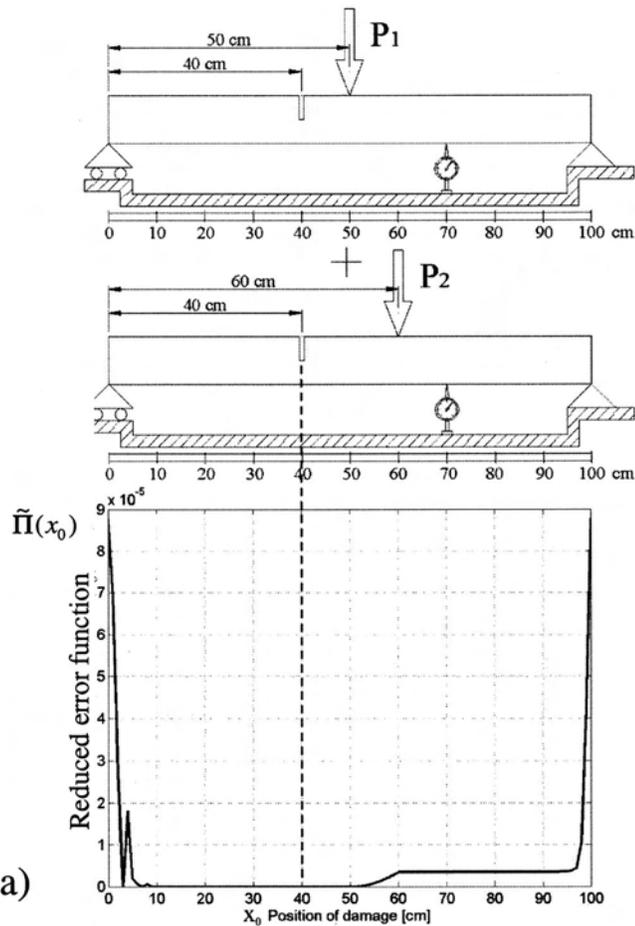
**Fig. 10.** Pinned-pinned beam with a single damage, one deflection measurement, and two concentrated load conditions on one side of crack: (a) reduced error function  $\tilde{\Pi}(x_0)$ ; (b) error function  $\log \Pi(\alpha, x_0)$  with its contour lines
