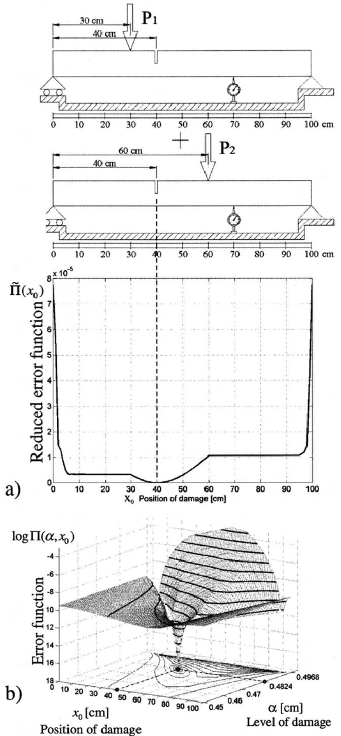
Fig. 9. Pinned-pinned beam with a single damage, one deflection measurement, and two concentrated load conditions bridging the crack: (a) reduced error function  $\tilde{\Pi}(x_0)$ ; (b) error function  $\log \Pi(\alpha, x_0)$  with its contour lines
