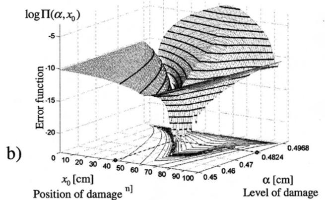
**Fig. 2.** Pinned-pinned beam with a single damage and two deflection measurements bridging the crack: (a) reduced error function  $\tilde{\Pi}(x_0)$ ; (b) error function  $\log \Pi(\alpha, x_0)$  with its contour lines
