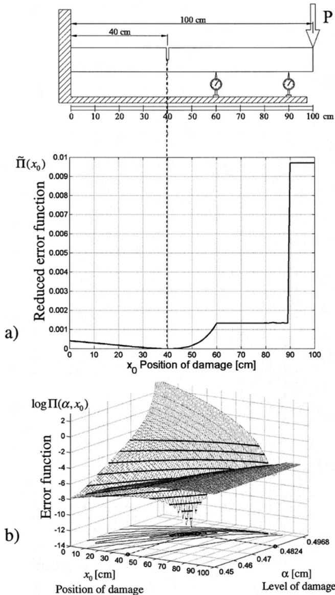
Fig. 8. Clamped-free beam with a single damage and two deflection measurements on the right of the crack: (a) reduced error function  $\tilde{\Pi}(x_0)$ ; (b) error function  $\log \Pi(\alpha, x_0)$  with its contour lines
