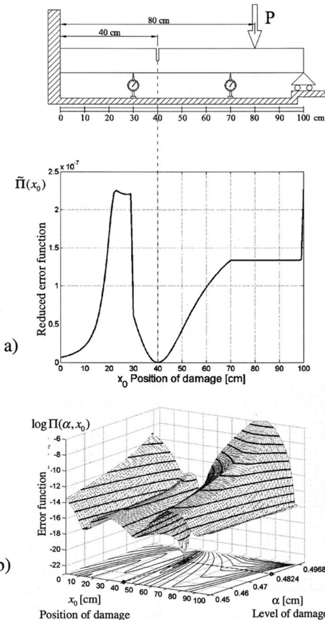
**Fig. 4.** Clamped-pinned beam with a single damage and two deflection measurements bridging the crack: (a) reduced error function  $\tilde{\Pi}(x_0)$ ; (b) error function  $\log \Pi(\alpha, x_0)$  with its contour lines
