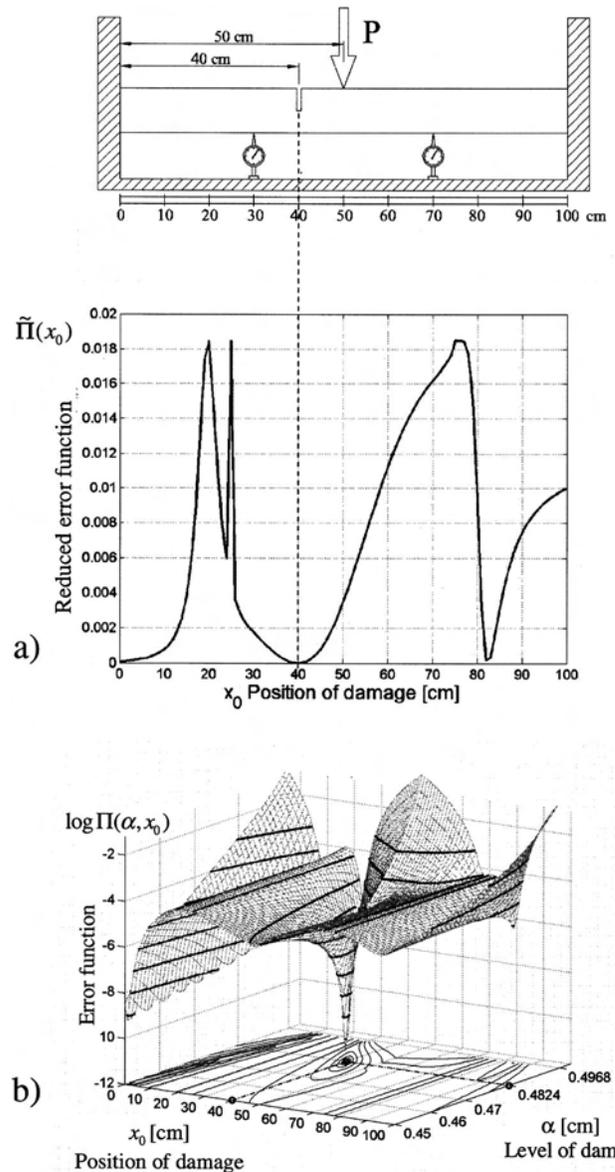
**Fig. 5.** Clamped-clamped beam with a single damage and two deflection measurements bridging the crack: (a) reduced error function  $\tilde{\Pi}(x_0)$ ; (b) error function  $\log \Pi(\alpha, x_0)$  with its contour lines
