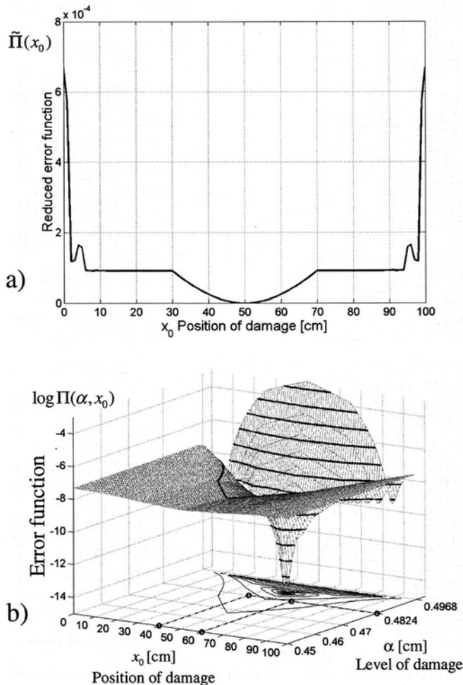
**Fig. 14.** Pinned-pinned beam with double damage and two deflection measurements: reduced error function  $\tilde{\Pi}(x_{01}, x_{02})$  evaluated by means of the model with a single crack
