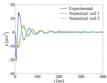
Figure 8. Numerical versus experimental acceleration history.
