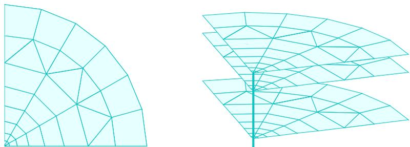
Figure 6. BEM discretization of the pile-soil system.
